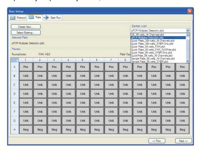
12.3.4. On the Plate Editor Screen, change the Sample Type to correlate with your specific plate setup. NOTE: To select the Sample Type, highlight the wells you would like to define, then choose from the dropdown menu one of three types:
