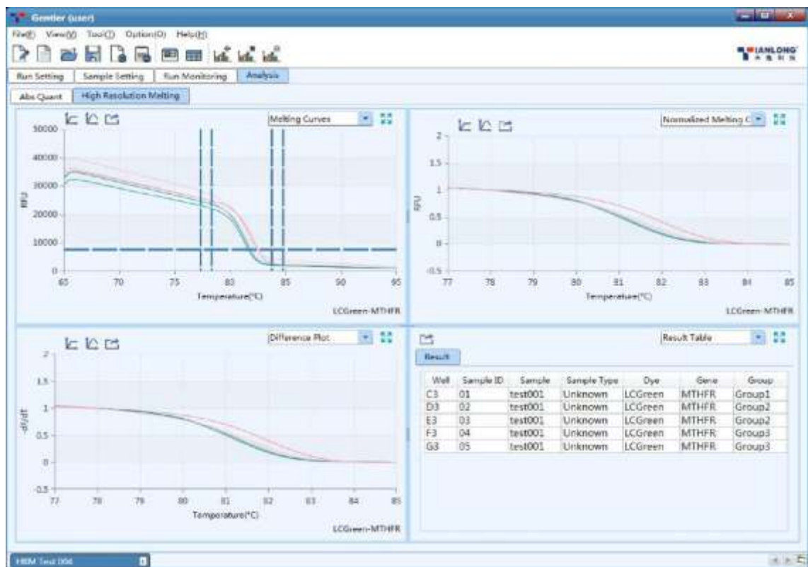
Figure D-14. High Resolution Melting analysis interface
