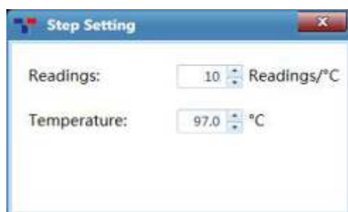
Figure D-5.6f Step Setting Dialog Box – Continuous Melting Step Mode
