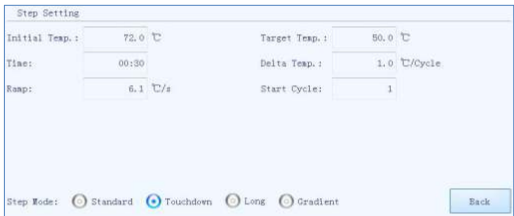
Figure E-3.5 Temperature Setting sub-tab - Step Edit window - Touchdown step mode
