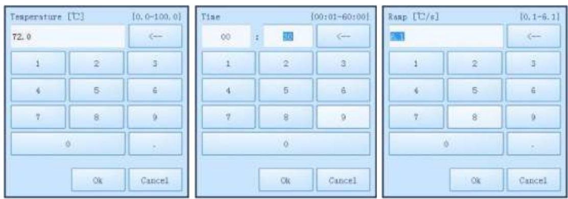
Figure E-3.4a. Step Edit window - Standard step parameter setting
