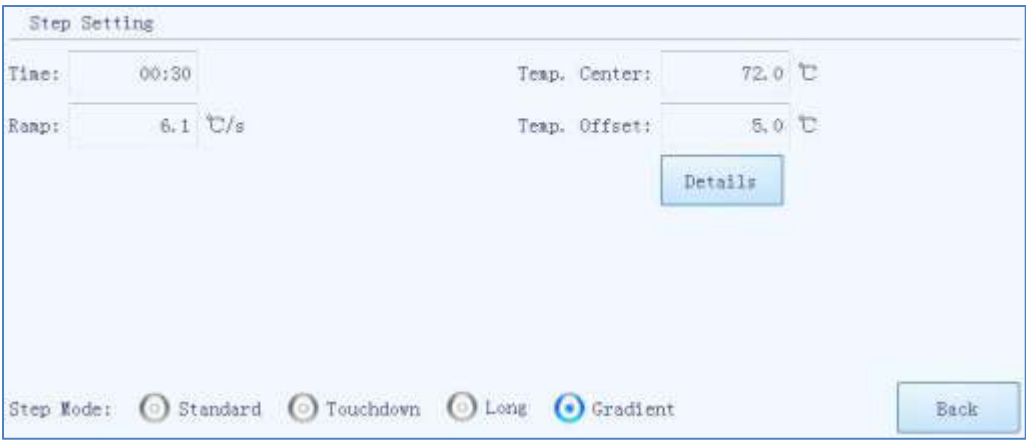
Figure E-3.7 Temperature Setting sub-tab - Step Edit window - Gradient step mode
