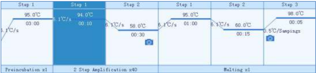
Figure E-3.1 Temperature Setting sub-tab - Example temperature program
