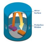
CO2 Incubator Dual Wave Infrared (IR) Sensor
