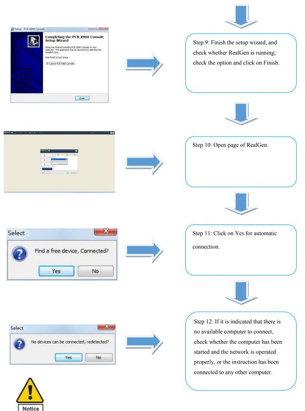
If the instrument connection fails, check whether it has been properly connected to the computer; if yes, shut down any anti-virus software and restart the instrument, and then try connection after it beeps. If connection fails again, contact the dealer for a solution.
